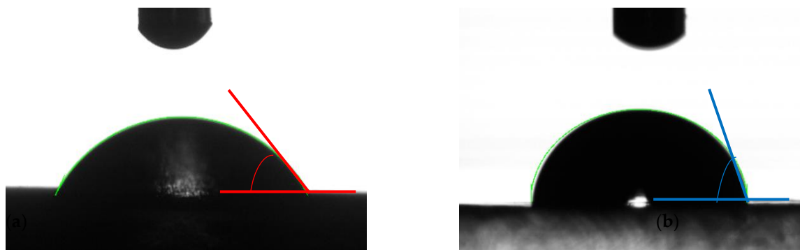
Figure 3-24: Image of water drop onto the surface of PLA (left) and TPU (right).
