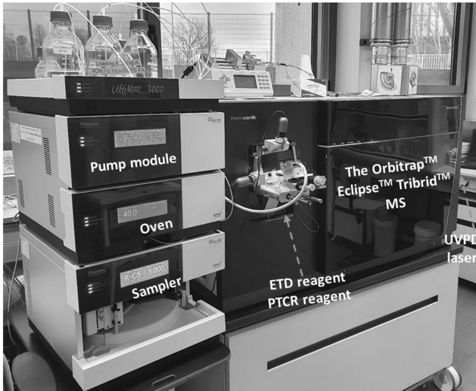
Picture of the the Ultimate™ 3000 LC coupled to The Orbitrap™ Eclipse™ Tribrid™ MS (Thermo Fisher Scientific, USA)
