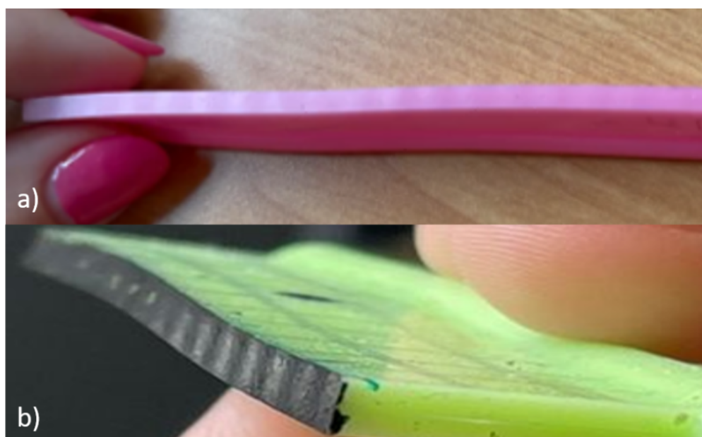
Figure 3.19: Patterns on the surface of elastomers a) E8 and b) E32 with an applied strain of 20% after cutting by blade 3 at a speed of 1 mm/s.
