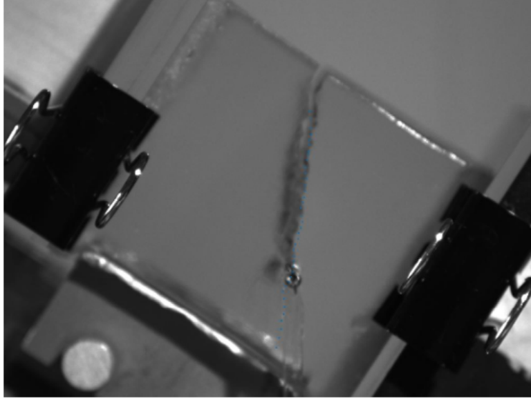
Figure 4.18: Propagation of the crack tip (dots) in gelatin gels subjected to a 2% applied strain using a 14g weighted wire, with approximation curves (lines).
