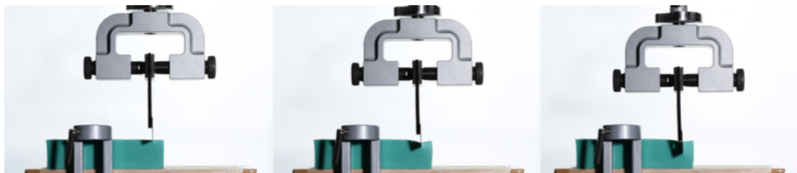
Figure 5.7: The stiffer holder bending during the experiment, leading to angled cuts. The sequence shows: 1) the position of the blade before contact with the sample surface, 2) initiation of the cutting, and 3) cutting in progress. .
