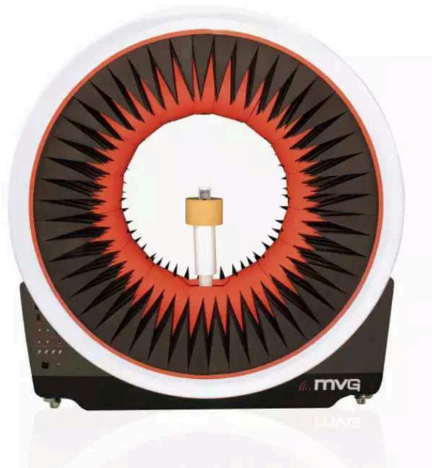
Figure 1.10: Starlab near-field range (Max. weight of DUT of 15 kg and dimension of 45 cm in diameter) [42]
