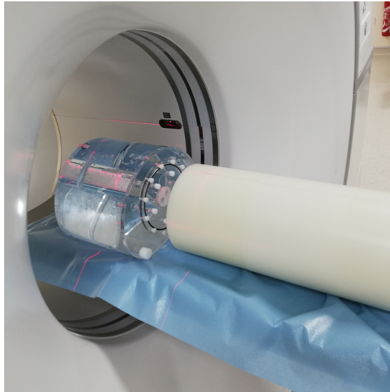
Figure 9.7: Image of the NEMA IEC phantom on the DMI patient bed. The NEC phantom was placed on the patient bed outside the FOV.
