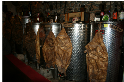
Figure 1.2: Wine fermentation in stainless steel tanks [53].
