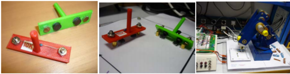
Fig. 1.10 On the left: the DUT components equipped with magnets; On the right the robot placing a component on the board.
