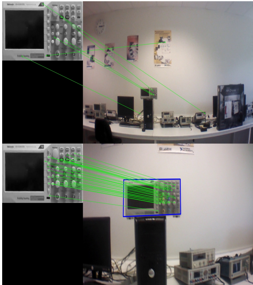
Fig. 3.5 Object detection using the SIFT approach with different distance from the object. On the left the template image of the object to detect, on the right the current image. Green rays are correspondence points.
