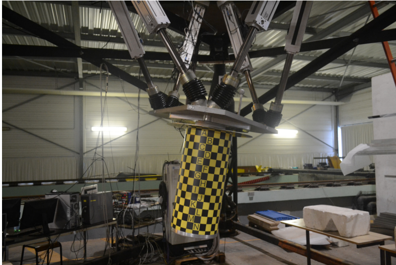
Figure 5.19 – A moving cylinder in the air (outside of the wave tank) to measure the inertia loads.
