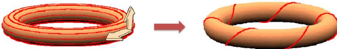
Figure 1.5: Magnetic fields in both poloidal (vertical) and toroidal (horizontal) directions are at the foundations of the tokamak concept.
