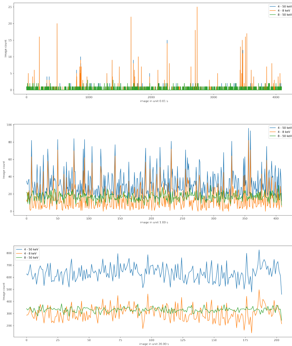
Figure 5.5: From top to bottom, lightcurve figure of TVAC test in 10 ms, 1.0 s, 20 s time-bin in different energy bands.
