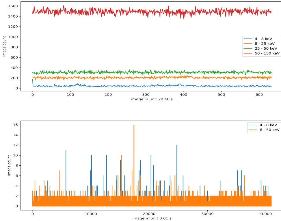
Figure 5.26: Top: lightcurve of the detection plane in the TVAC test conducted in Shanghai on September 28, 2023. This part of the figure illustrates the lightcurve over a duration of 12963.84 seconds. Bottom: a selected segment of the lightcurve spanning 400 seconds, divided into 10 ms time-bins.
