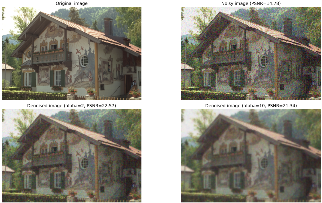
Figure 3.1 – Results of denoising an image by minimizing the variational cost of equation 3.3 through automatic differentiation, with two values of \alpha .
