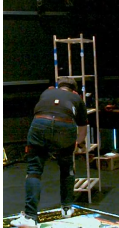
Figure 2.3 – Illustration of auto-occlusions of the left arm with a camera positioned behind the subject for the work task
