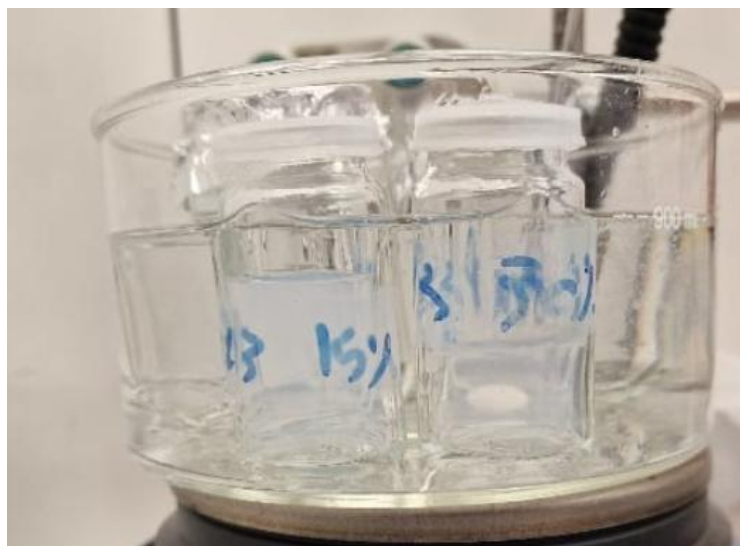
Figure IV-S8. Physical aspect of P123-MA solutions at 15% w/w (left) and 30% w/w (right) when heated to 70 °C.
