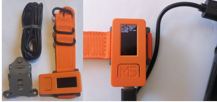
Figure 5.22: The mini-ESP32 M5StickC IoT devices used in the experiments
