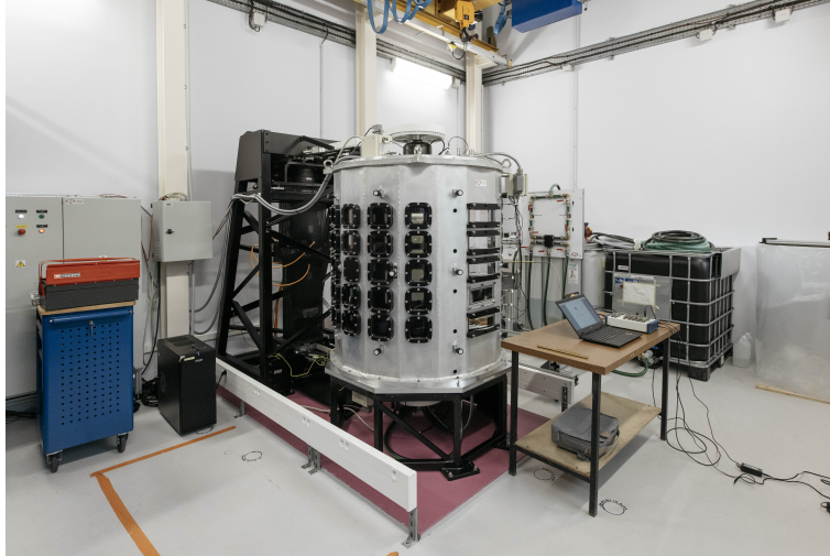
Figure 8.1: Picture of the 'Giant Von Kármán' experiment. The black motors on the left drive the belts above and below the aluminium case, rotating the impellers inside.
