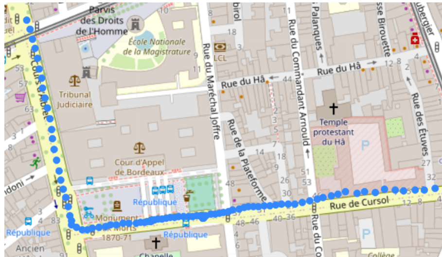
FIGURE 5.1: An example of the trajectory that was extracted from CAM messages, plotted on top of an OSM map
