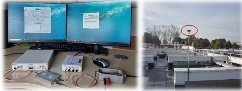
Figure 4.9: GNSS Signal Recording System and MATLAB-based Jammer (Left) connected to an antenna mounted on the roof of the building (Right).
