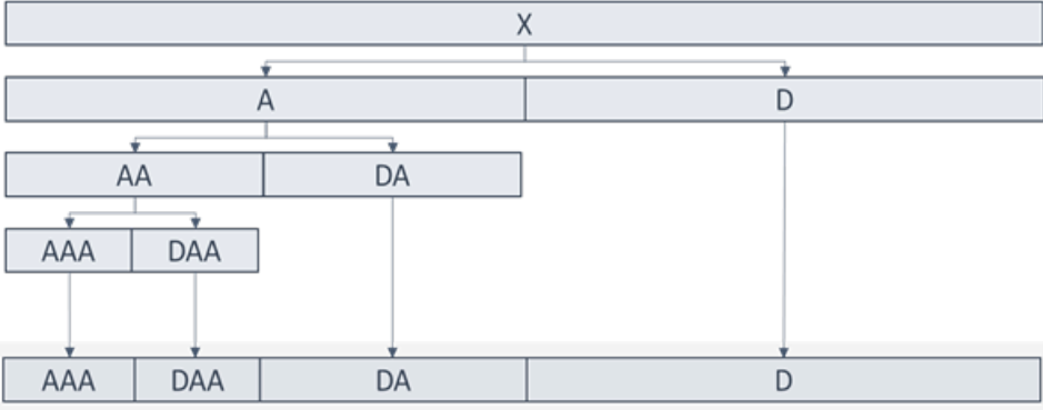
Figure 4.20: A three-level discrete wavelet decomposition (dwt); approximation (a) and detail (d) block represent the lowpass and highpass filtering and the subsampling operation
