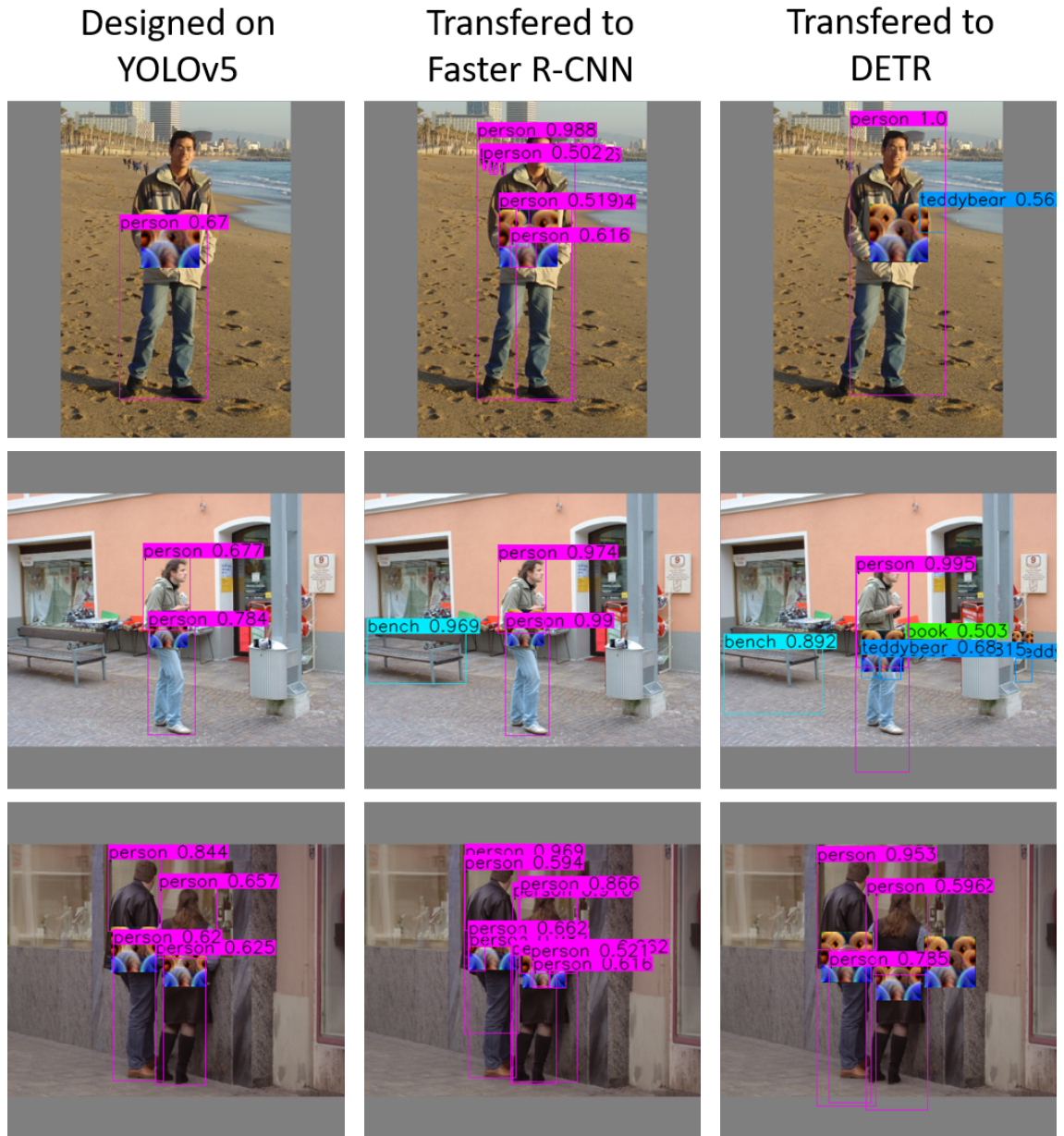
Figure 5.1: Examples of white-box (designed on YOLOv5 and applied to it) and black-box transfer invisible cloak attack. The patch is designed on YOLOv5 and is from Huang et al. (2023) work. Patches are designed to prevent persons from being detected.
