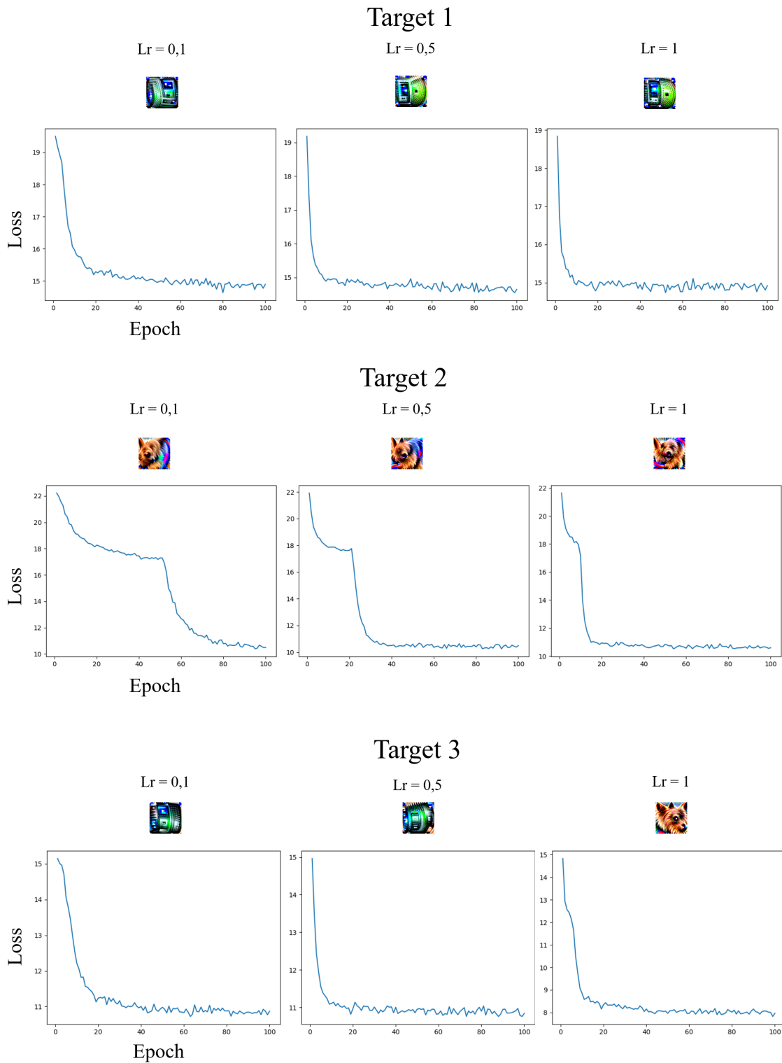
Figure C.2: Learning curves and resulted patches of the L2 method for different targeted points. For each targeted point the optimization is run for three different learning rate. The source model is ResNet50-v1 and the targeted class is Australian terrier.
