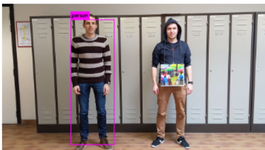
Figure 2.21: Two examples of real-world footage perturbed by an adversarial patch attack. The person wearing the patch is hidden from the object detector while the other is detected. The authors provided a demonstration of their attack here . Source: Thys et al. (2019)
