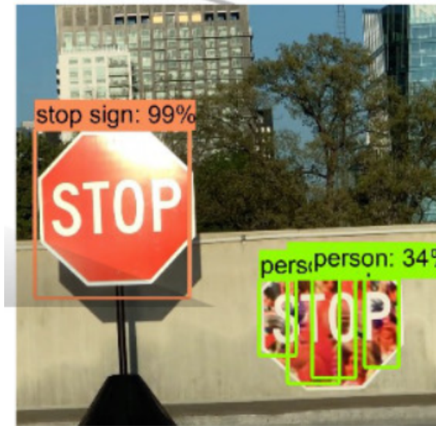
(b) Example of the stop sign targeted attack in real-world conditions. The APA is designed to sway the detector to output another class, here person . The unattacked left stop sign is correctly detected, while the attacked one on the right is detected as person . Source: Chen et al. (2019)
