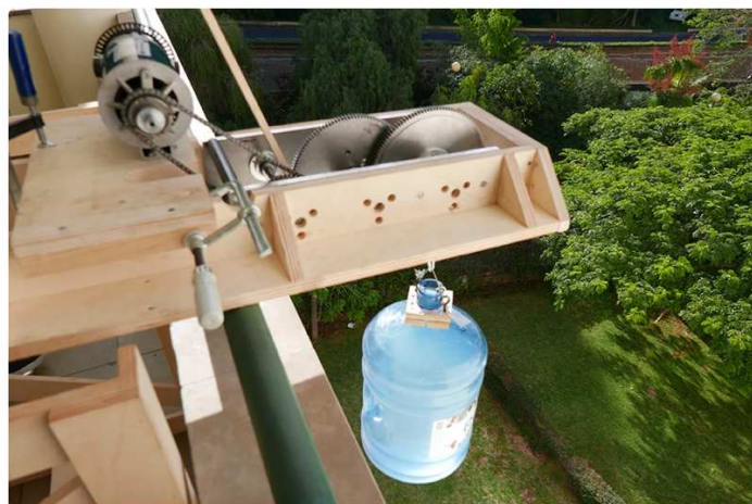
Figure 30. Gravity Battery from Auger et al. (2019). It uses a combination of natural and cultural materials to generate and store energy, thus helping to raise awareness about our current unquestioned energy consumption.
