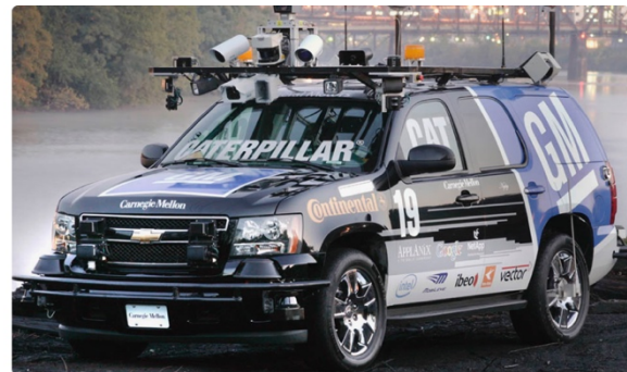
Figure 10. Left: The winning Stanley VW Touareg from Stanford Artificial Intelligence Laboratory (DARPA Grand Challenge of 2005). Right: The winning Chevy Tahoe "Boss" from Carnegie Mellon University and General Motors (DARPA Urban Challenge of 2007).
