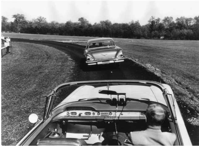
Figure 8. Left: Autonomous Highway System tests from General Motors (GM) and Radio Corporation of America (RCA), 1950. Right: "Electricity may be the driver" ad in the magazine Life in January 30, 1956.
