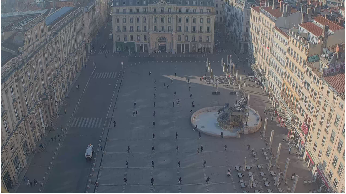
FIGURE B.3: Image used for calibration, reconstructed from excerpts of a LargeView camera footage at Place des Terreaux in 2023. I positioned myself at each node of the square lattice marked on the ground, where each square has a side length of 640 cm.
