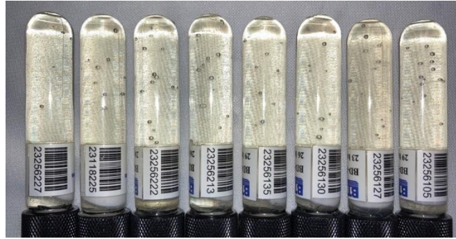
Figure 3.7 – Bubble detectors used during the experiment. Eight BD-PND were placed simultaneously at the same position to increase the total number of bubbles produced and reduce the statistical error.
