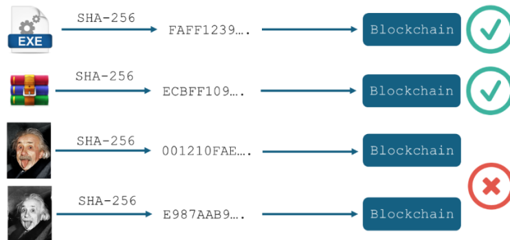
Figure 6: Blockchain solutions are design to detect any modification in the recorded content, regardless of its impact in the content semantics
