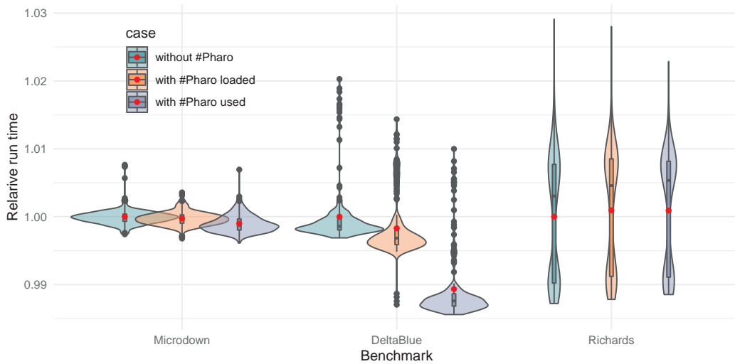
Figure 7.1: Relative run time performances with global cache disabled on Microdown, Deltablue, and Richards benchmarks. Lower is better. A red dot marks the average.
