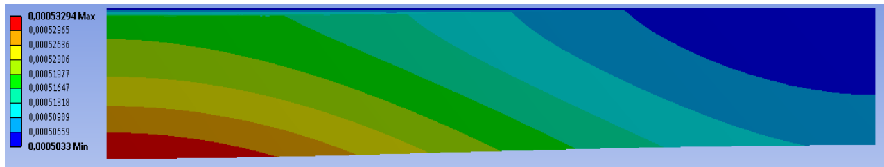
Figure 86: total deformation of the target (m). The scale is amplified (8.7x).
