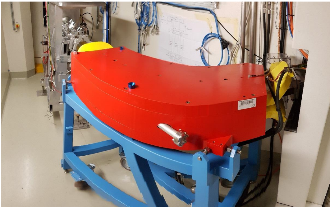
Figure 30: magnet of the MEDICIS mass separator in its dedicated bunker. Only the exit line at 0° is used.
