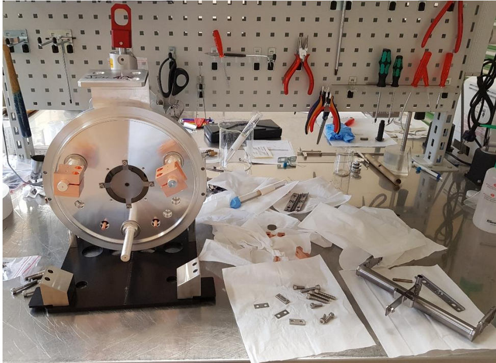
Figure 29: ISOLDE/MEDICIS target unit assembling. On the left the predefined base; in the middle tantalum components; on the right the target container and surface ion source.
