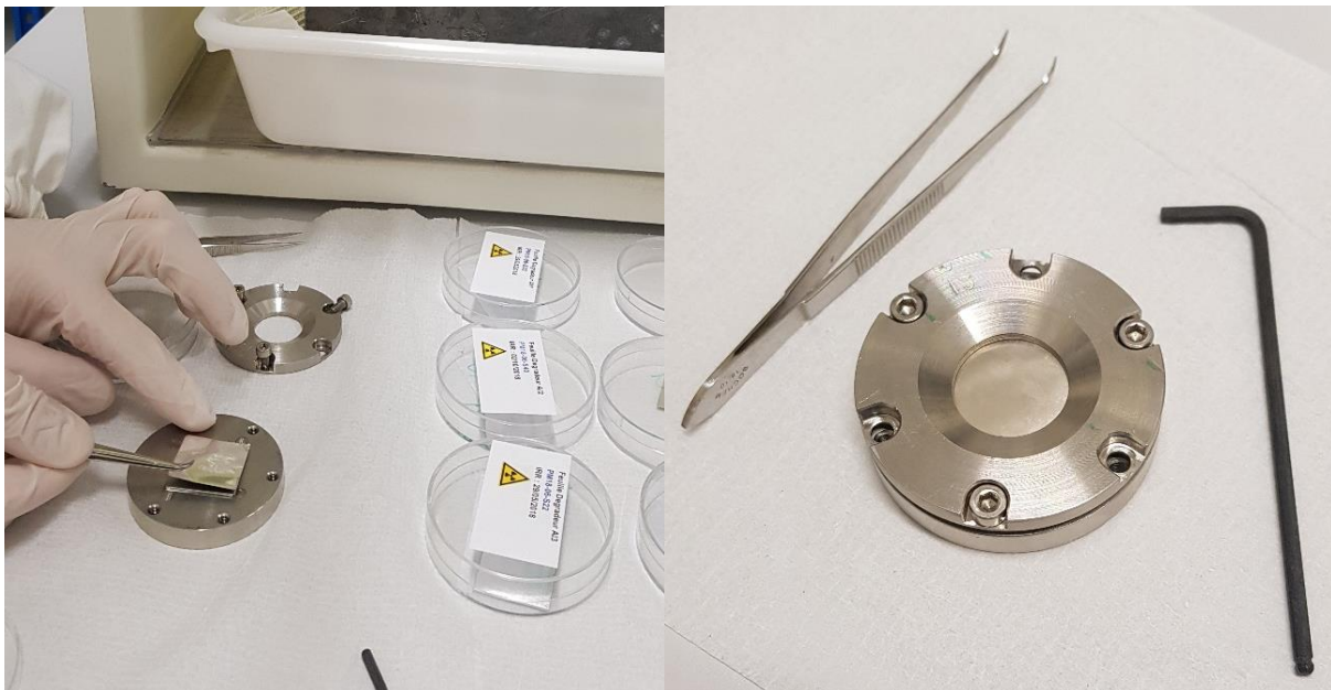
Figure 44: preparation of the stacked foils, on the left the stack assembling, on the right of the mounted stacked which will be irradiated
