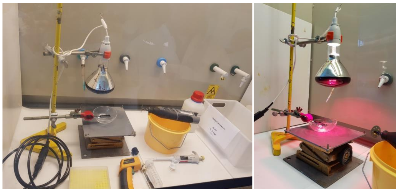
Figure 91: on the left the experimental setup in the fume hood at Hevesy Laboratory (DK). On the right the evaporation of the erbium acid solution for the deposition on the graphite support
