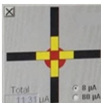
Figure 3.3: Dynamic operator interface of particle depositions on each fingers of the collimator.
