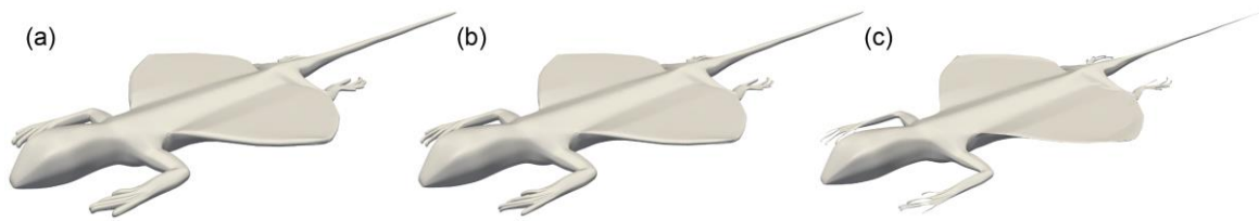
Figure 5-4: Geometries used in sensitivity analyses to assess the impact of geometry construction: (a) bulkier P0 geometry; (b) preferred P0 geometry; (c) thinner P0 geometry.
