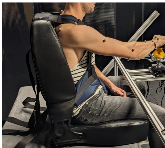
Figure 5.2: The shoulder and abdomen strips ensure a straight back. The shoulders translations are also strongly limited in range, in order to allow only rotations.
