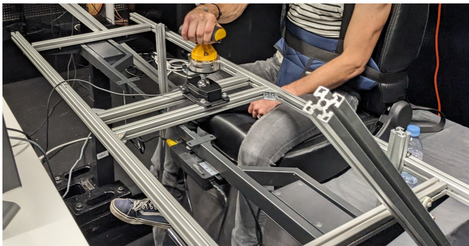
Figure 5.5: This adjustable custom-made aluminum profile support allows for precise positioning of the force/torque sensor to accommodate participants of different sizes and varying upper limb postures.
