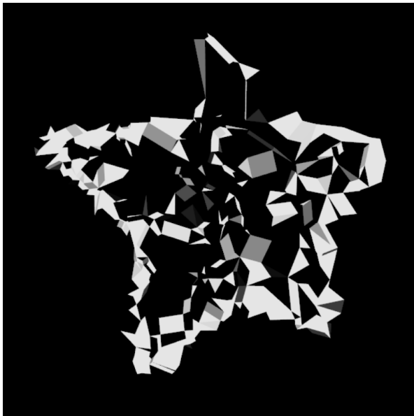
(a) Reconstruction on a coarse mesh. The central slices of the volume were reconstructed on an unsuited mesh. The size of the tetrahedra needs to be reduced.
