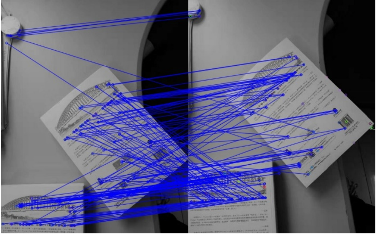
Figure 3.4: Results of the correspondences found by the SIFT algorithm between two images [5].
