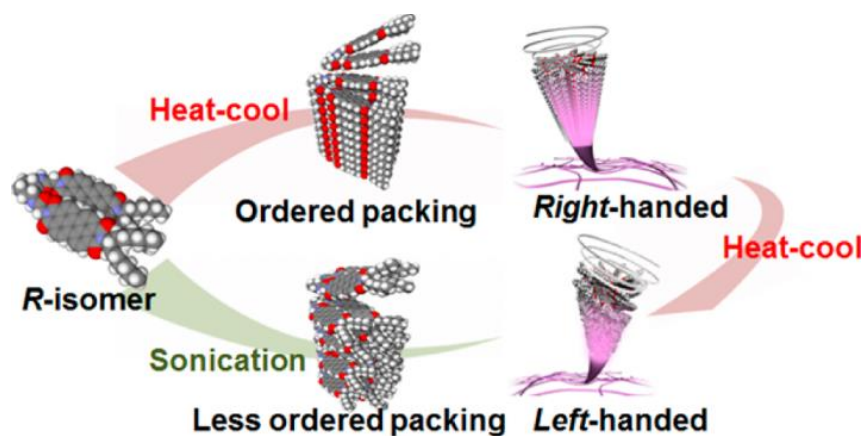
Figure 31 | Schematic representation of the structural differences according to the method of preparation that lead to the reversal of supramolecular chirality. (Reproduced from 76 ).
