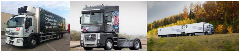
Figure 1.4: Rigid on the left, Tractor on the middle, Rigid and trailer on the right.
