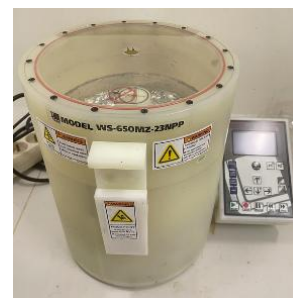
Figure 27. A spin-coating machine is used to deposition the transporting layer under ambient conditions.
