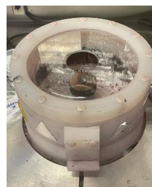
Figure 28. A spin-coating machine is used for the active layer in the glove box.
