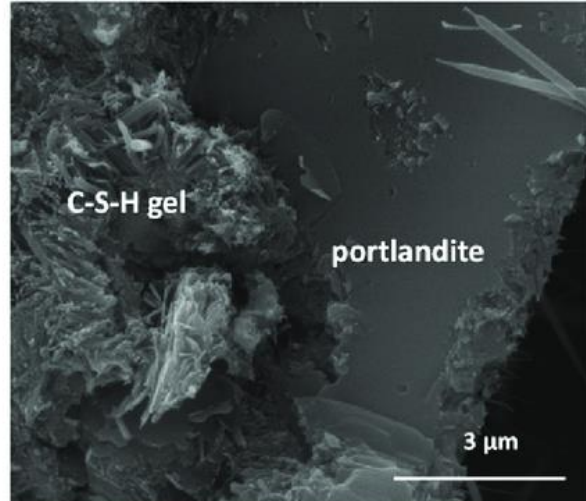
Figure 52: SEM observations of portlandite crystals in Portland and blended cement [195].
