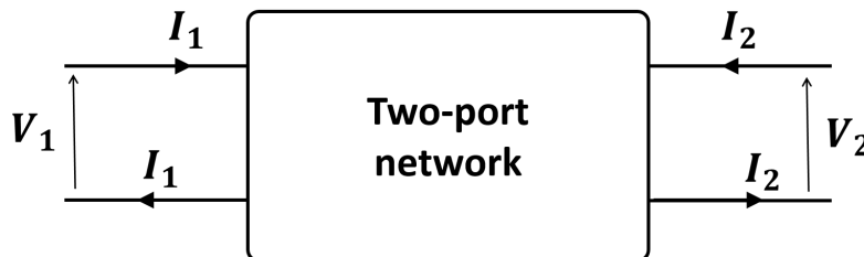
Figure 2.1: Representation of a two-port network
