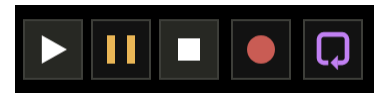
Figure 2.8: From left to right: the sc-transport element in the "pause" state, the sc-record in the active state, the sc-loop component in the active state.
