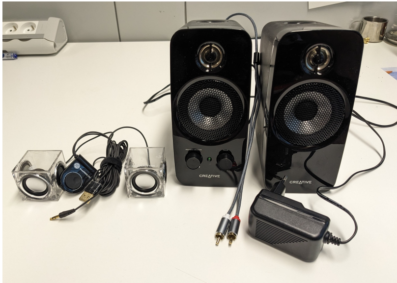
Figure 7.3: Two types of loudspeakers used. On the left: GOgroove Son-aVERSE CRS speakers. On the right: Creative Inspire T10 speakers.
