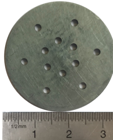
Figure 6.8: Front view of the optimised circular plate
