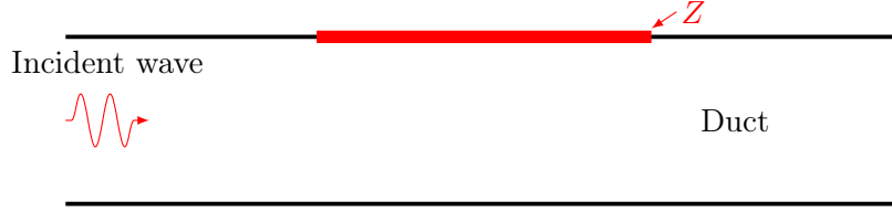
Figure 3.2: Sketch of the duct with surface impedance modelling
