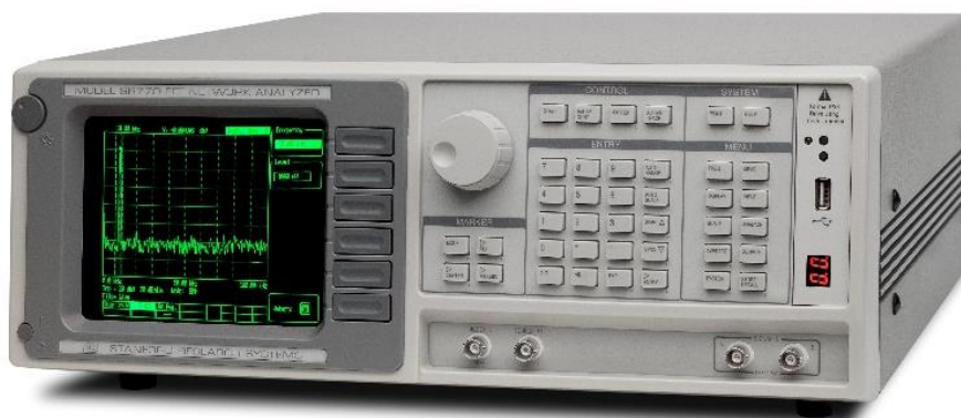
Figure 2.15 – Spectrum analyser (Stanford Research Systems SR770)
