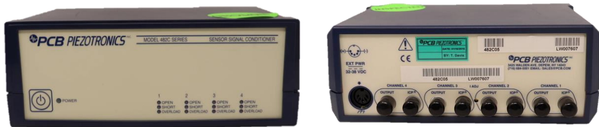
Figure 2.20 – Signal conditioner (PCB 482CXX) front panel (left) and rear panel (right)
