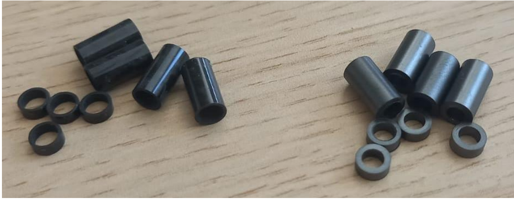
Figure 4.24 – Composite material insulating spacers and washers, in CFRP (left) and Vespel SP22 (right)
