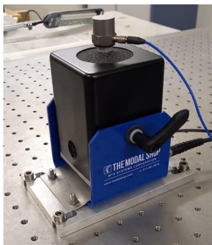
Figure 2.23 – Mechanical shaker mounted on optical bench &amp; accelerometer mounted on shaker moving part
