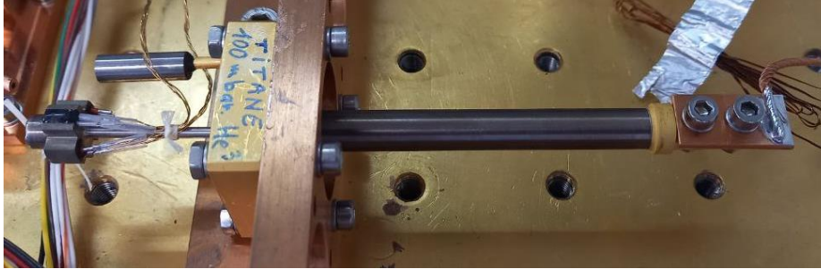
Figure 0.2 - Gas-gap heat switch (main test object)
