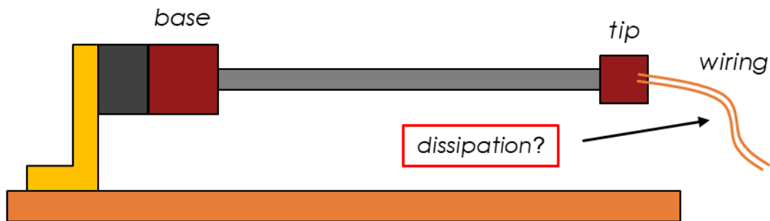
Figure 4.33 – Hypothesis: dissipation is occurring in wiring of heat switch tip instrumentation
