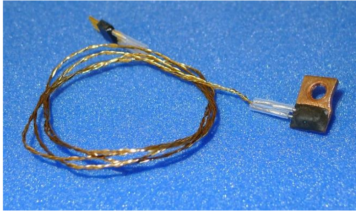
Figure 2.29 – Electrical heater (Vishay) with copper fixing plate
