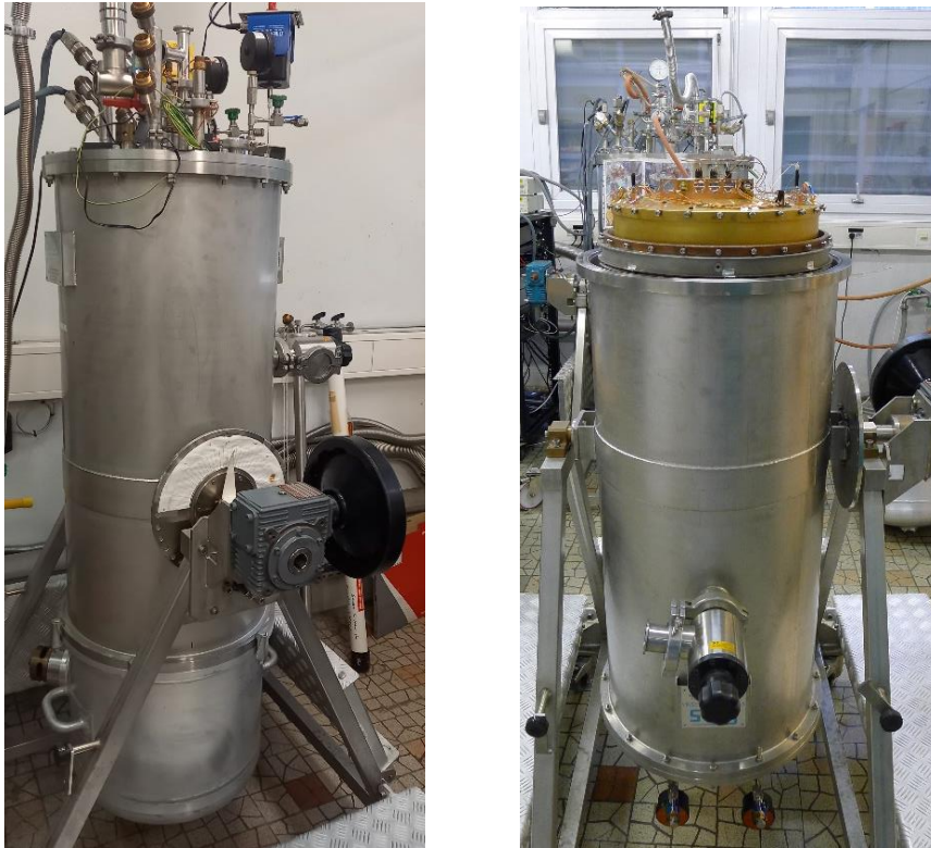
Figure 2.9 – Herschel cryostat in the upside down position closed (left) and upright position open (right)
