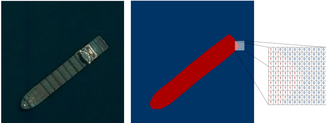
Figure 1.11: Semantic segmentation applied to ship detection. Class 0 (■) corresponds to background pixels, and class 1 (■) to ship pixels.
