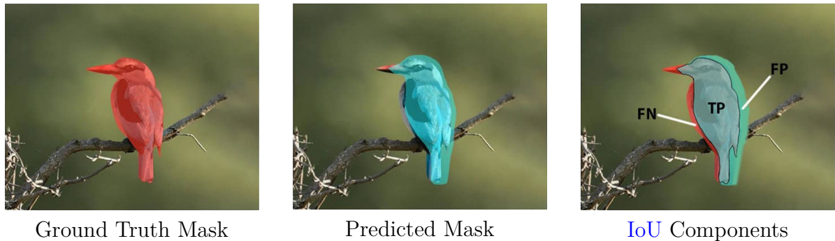
Figure 1.12: Illustration of the different components used to compute the IoU metric and, in particular, the True Positives ( TPs ), False Negatives ( FNs ), and FPs elements.
