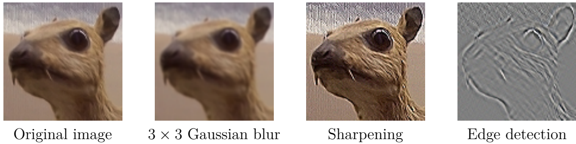
Figure 1.4: Examples of blurring, sharpening, and edge detection effects achievable by convolving kernels and images.
