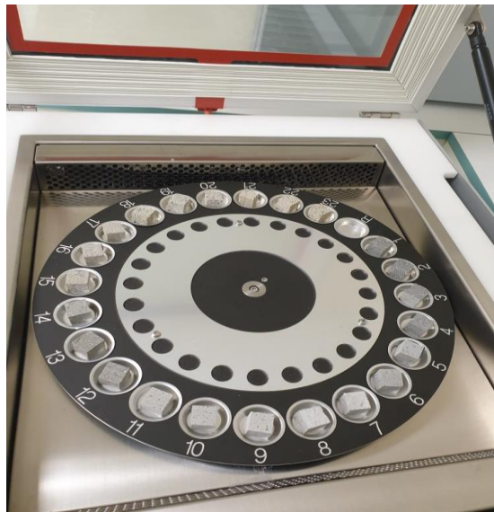
Figure II.44. Gravimetric vapor sorption analyzer (SPS model from ProUmid). Cubic mortar specimens are installed in the sample loader.
