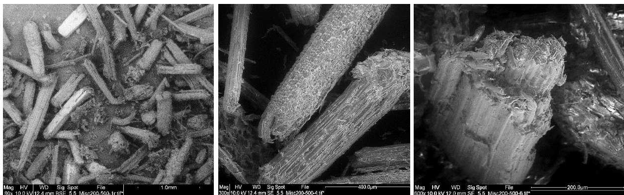
Figure II.40. Scanning Electron Microscopy (SEM) images of the micronized miscanthus fibers at different magnifications.
