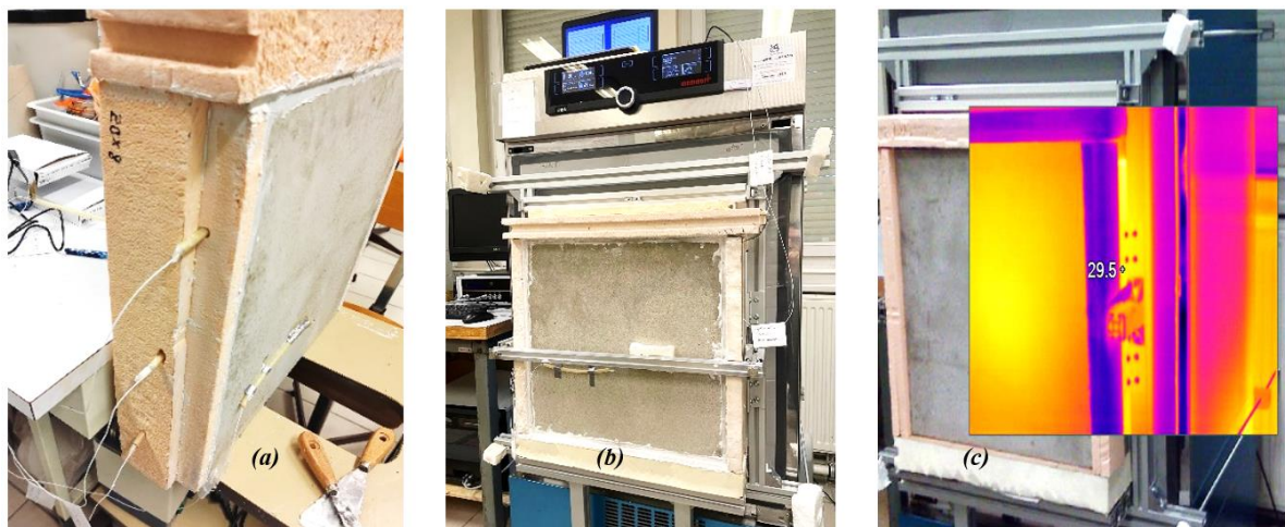
Figure III.2. (a) Wall preparation with sensors; (b) Experimental setup; (c) IR image of wall to check uniform heat transfer and to prevent the heat losses.
