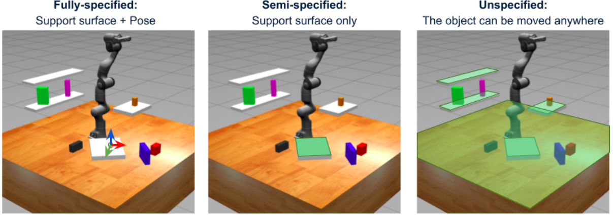
Figure 3.1: Visualization of the three types of goal specification. (a) Fully specified goal, (b) Partially specified goal, (c) Unspecified goal.
