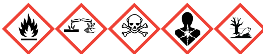
Figure I. 18 : Safety pictograms of Hz according to UN Globally Harmonized System (GHS) criteria
