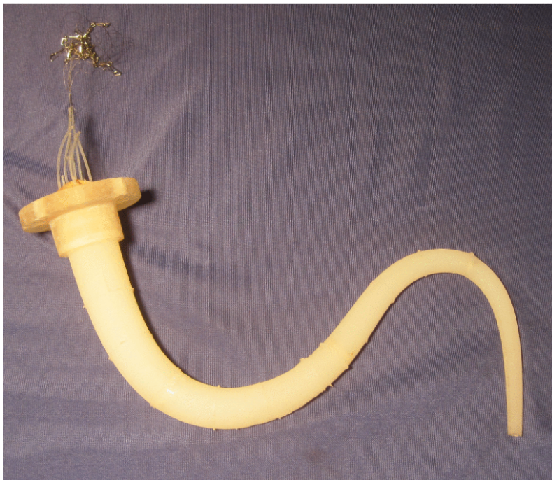
Figure 2.5: A multi-bending soft robot arm driven by cables [28].
