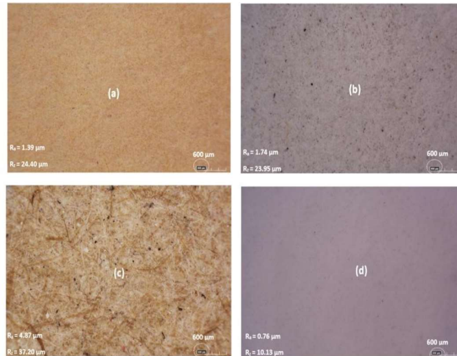
Figure 3.10 The surface roughness of different cardboard samples observed under the microscope (a) sample #1, (b) sample #2, (c) sample #3 (d) sample #4
