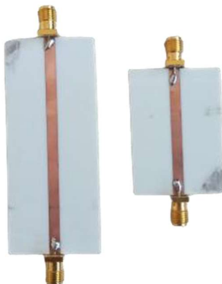
Figure 2: Image of fabricated Lines on RO4003C
