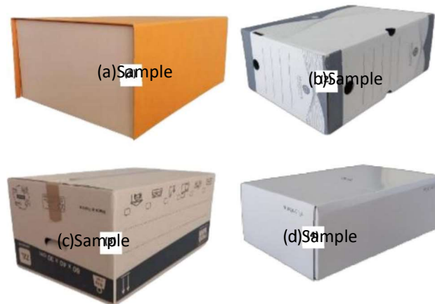
Figure 3.8: Different cardboard materials (a) sample #1 (2.2 mm) (b) sample #2 (2.15 mm) (c) sample #3 (d) sample #4
