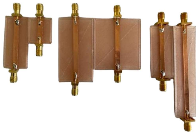
Figure 3.4:3D FDM printed substrat&transmission lines with copper tapes as conducting material
