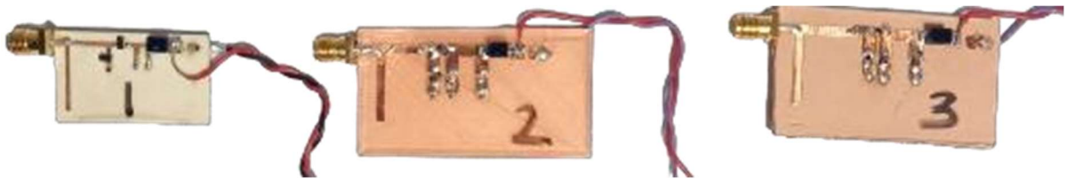
Figure 5.29: Identical rectifiers with three different (1) Rogers RO4003C, (2) PLA (3) Cardboard sample #1
