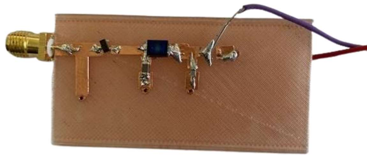
Figure 5.18: Picture of single series PLA base fabricated rectifier
