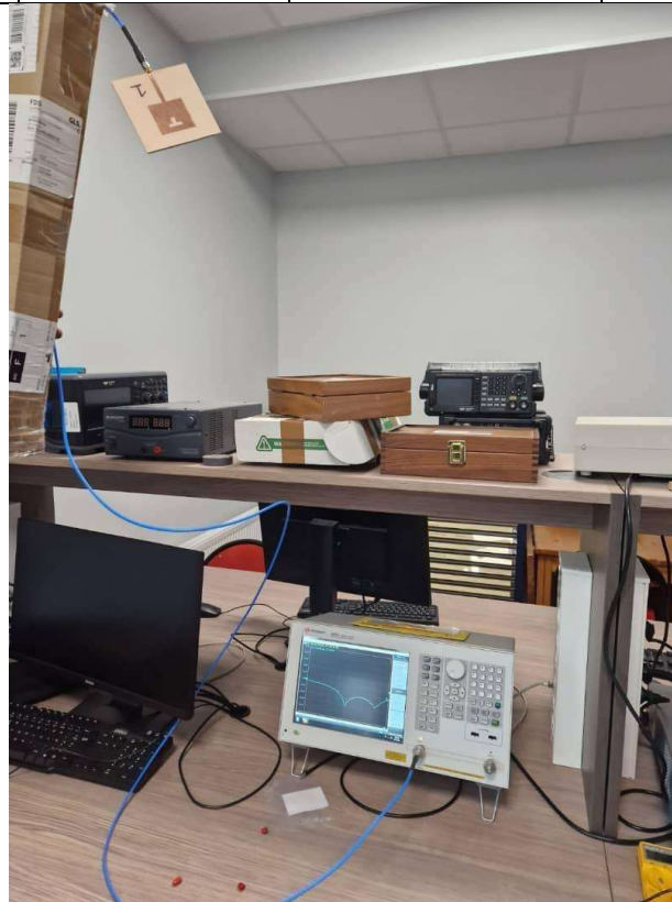
Figure 4.29: Lab setup for measuring return loss parameter of
