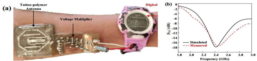
Figure 2.25: Flexible tattoo polymer antenna on PDMS support integrated with rectifier [88]
