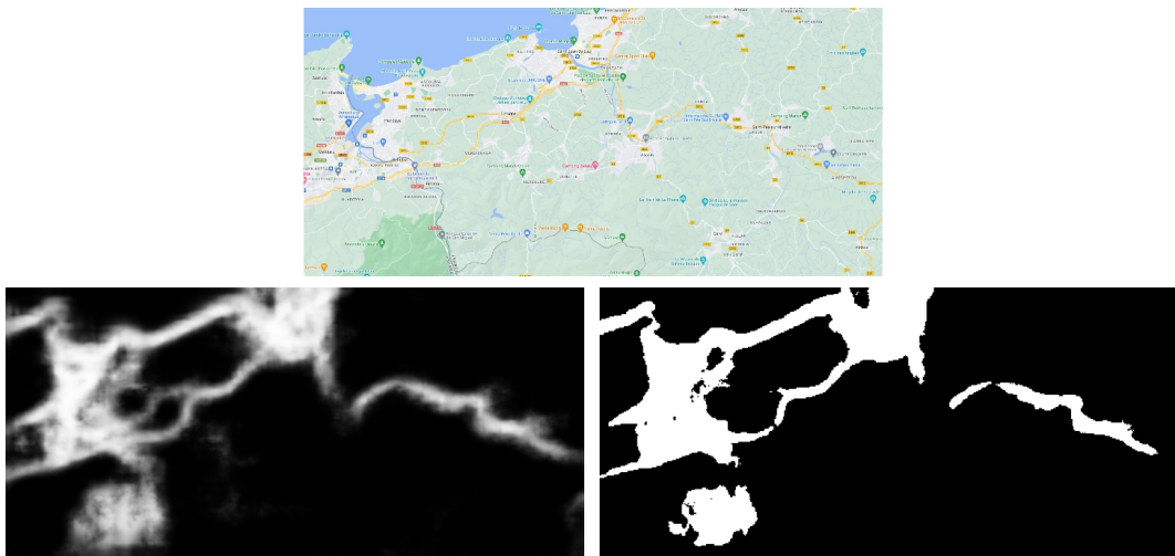
☼ Figure F.7 : Top: Original map image of Zone 2 from the evaluation dataset. Bottom left: Predicted AHAP probability heatmap from Segformer model. Bottom right: Corresponding binary segmentation map.
