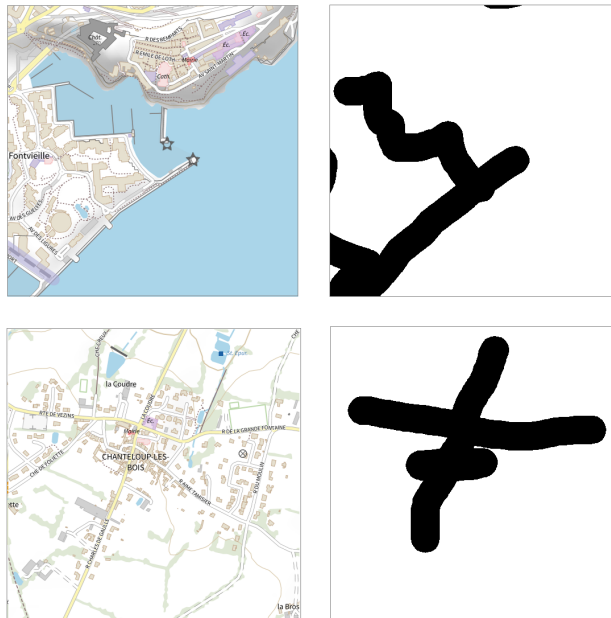
☞ Figure F.3 : Examples of tile/mask pairs extracted from the training dataset in order to train the U-Net model.
