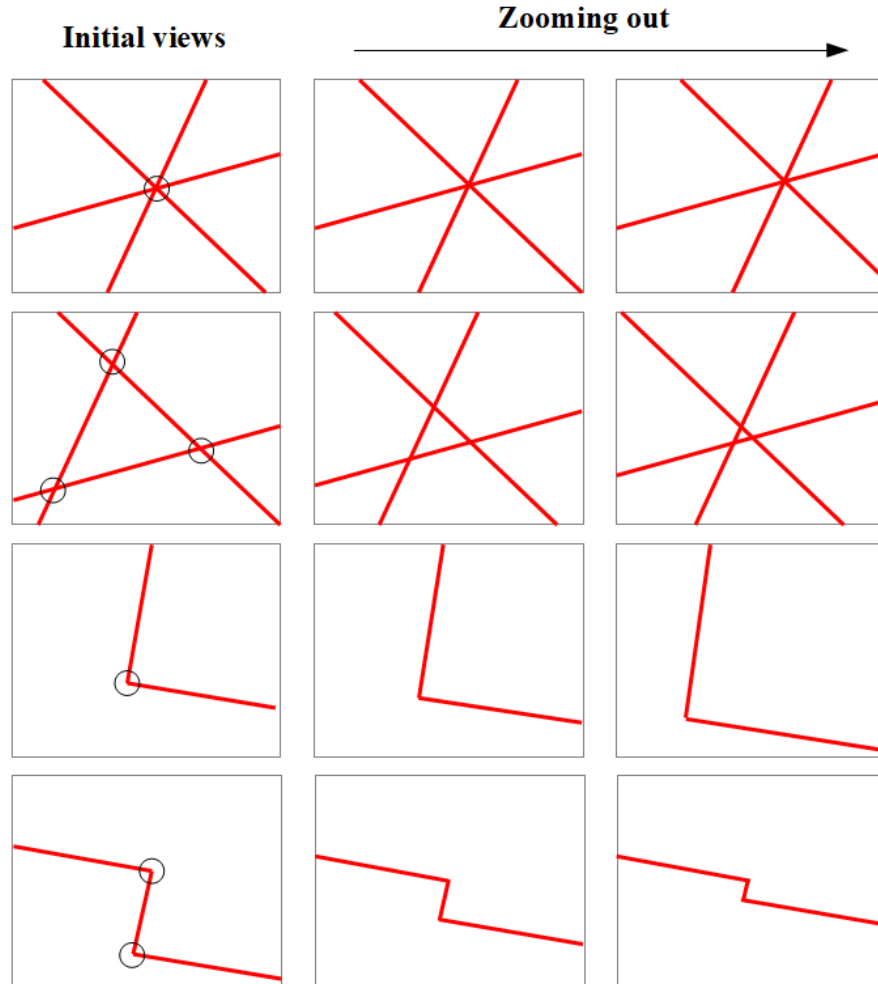
⌘ Figure B.5 : Intersections and bifurcations are what matters in order to indicate changes in scales, not the number of lines.
