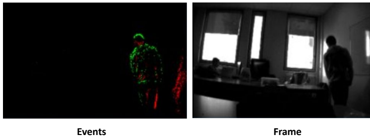
Figure 2.10: Event camera and standard camera output.
