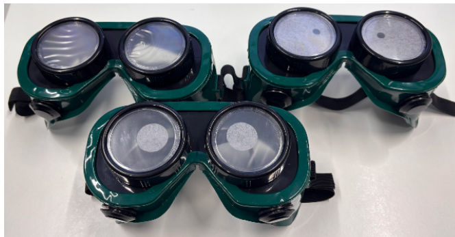
Figure 2.35: Simulation goggles used in this work (blurry vision top left, tunnel vision top right, central scotoma bottom)
