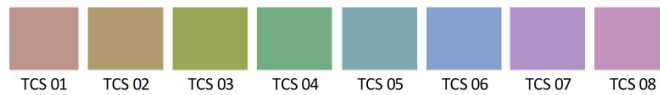
Figure 2.17: Test Color Samples (TCS) used for the calculation of the CRI R_a .
