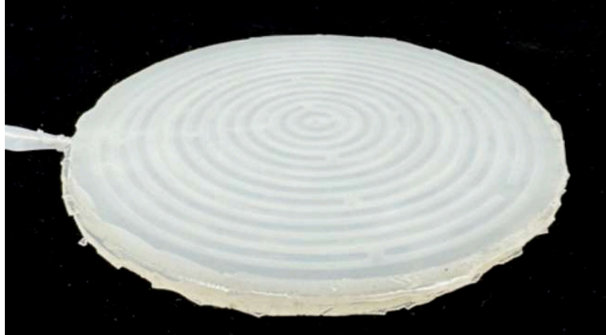
Figure 2.15: Baromorph made from silicone
