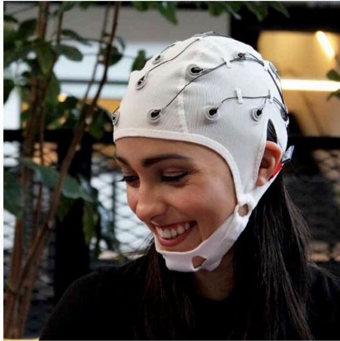
Figure 2.13: A 21-channel OpenBCI electrode cap kit (From [12])
