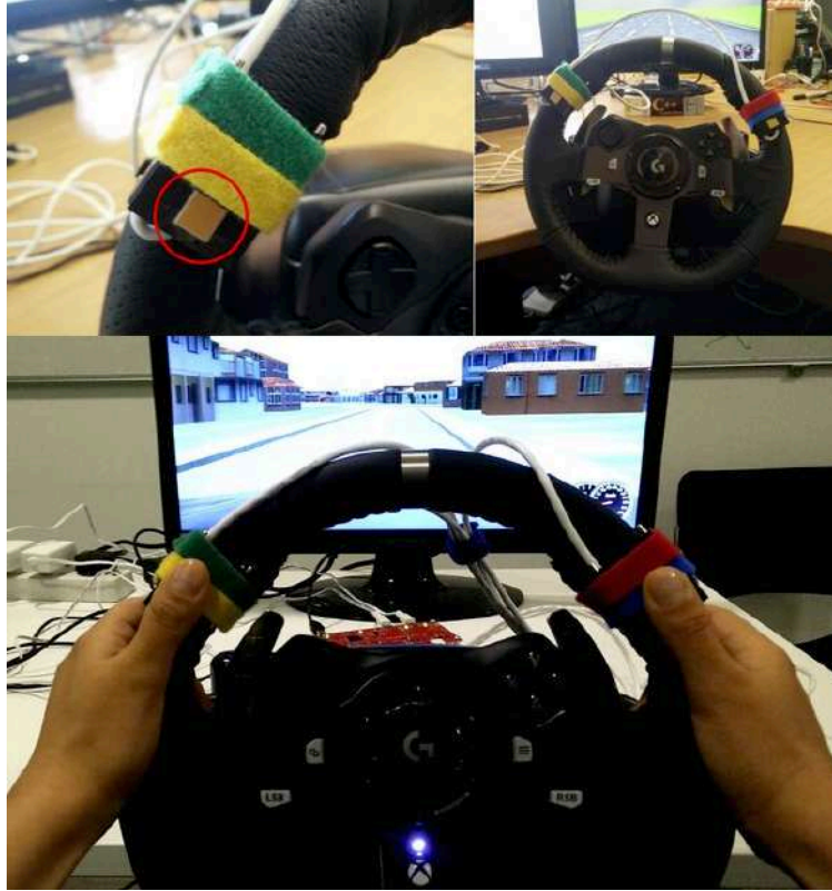
Figure 2.11: Thermal and Vibrotactile Notifications on the Steering Wheel (From [10]) Upper: Thermally-enhanced steering wheel with small Peltier elements; Down: The set-up of the navigation studies.
