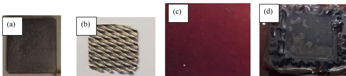
Figure 5.12. (a) Sintered Ti particles as PTL (1L flowfield), (b) course grid as flowfield, (c) homogeneous HNC membrane and (d) CCM after 73 h electrolysis using cell n°1.
