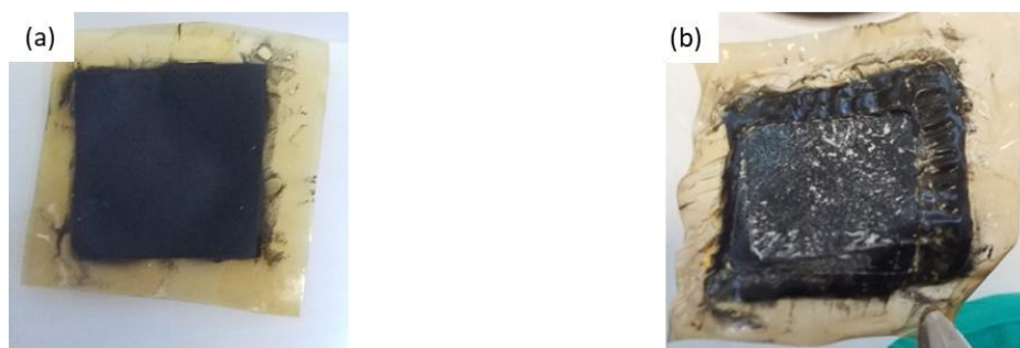
Figure 5.15. Images of HNC-CCM with HNC-180-2 membrane (a) before and (b) after electrochemical measurements.
