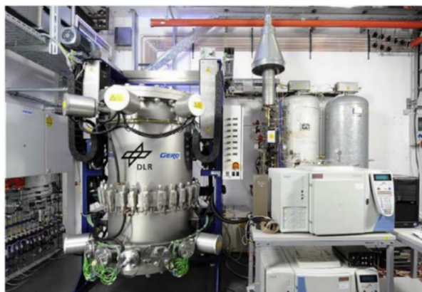
Figure 1.24. Pressurized solid oxide electrolysis cell (SOEC) stack test facility at German Aerospace Center (DLR) 45 .
