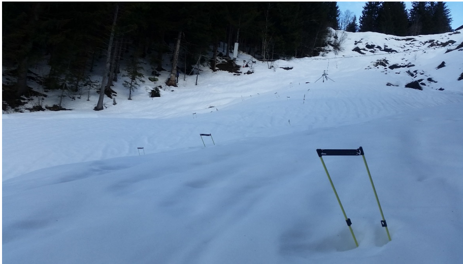
11. Photo illustrating the two main sources of inaccuracies in this experiment: the snow (the first snowfall) and the angle of the tag supports, which created a temporary error of (3\sigma) at the end of October and a slow drift roughly estimated at up to 5 cm per month, respectively. Apart from those two specific problems, the accuracy remained below 1.1 cm ( 3\sigma ).
