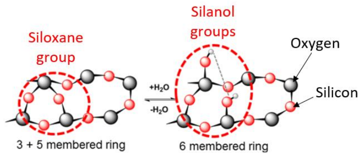
Figure 68. Hydroxylation of silica after exposure to humid environment: three- and five-membered rings opening to six-membered ring [120].
