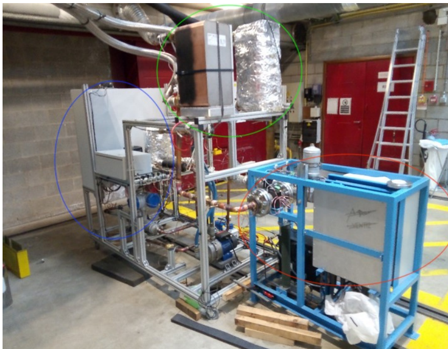
Figure A.1 – Coolant recovery test bench
