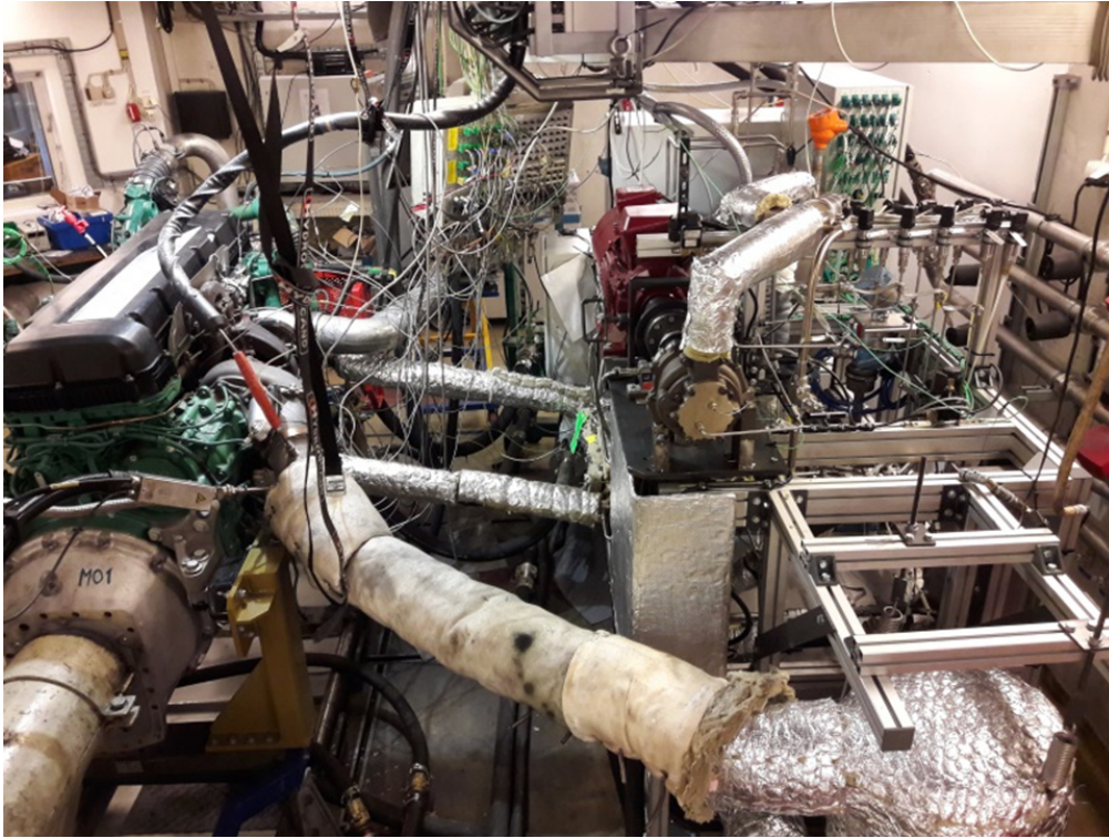
Figure 2.4 – Test bench in the Volvo facility in Lyon, widely used for model validation and testing of system architectures.
